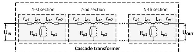
Figure 7: Equivalent circuit diagram of the cascade transformer.
